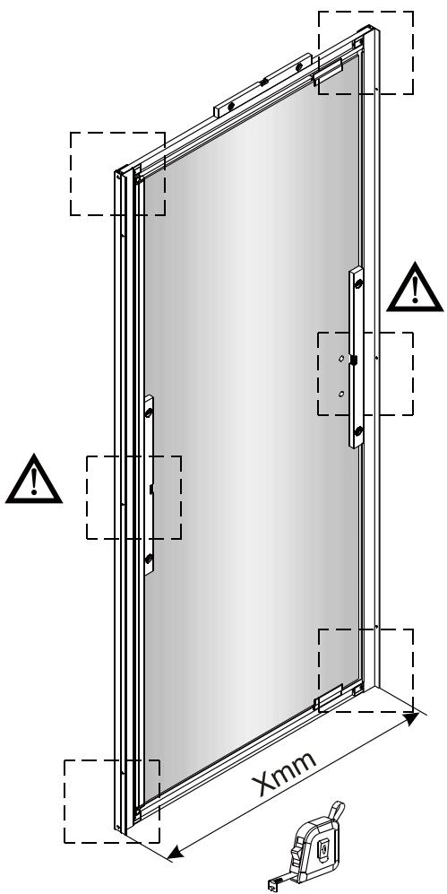
Note: When adjust the door, ONLY need to loosen the screw a little bit, DON'T loosen the screw completely.
