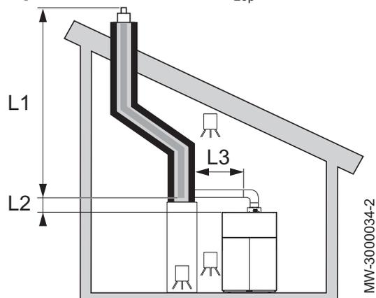
Fig.79 Fumisterie rigide B<sub>23p</sub>
