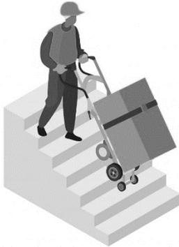
To move the water heater, use a hand truck and ensure that the inclination of the water heater does not exceed 45°.
