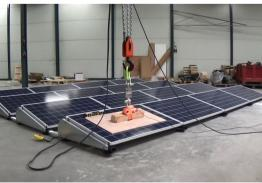
Based on mechanical lift tests carried out by Esdec with improved system connections in the summer of 2021, see right photograph up here, the actual degree of interconnection of the systems was determined and processed by us into the wind tunnel data. These have been
