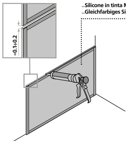
**Silicone in tinta Mapei ... Mapei coloured silicone sealant
