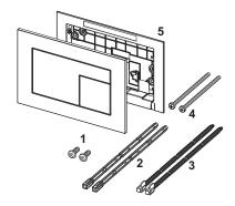
1 9820263 Fastening screws2 9820022 Actuation rods
