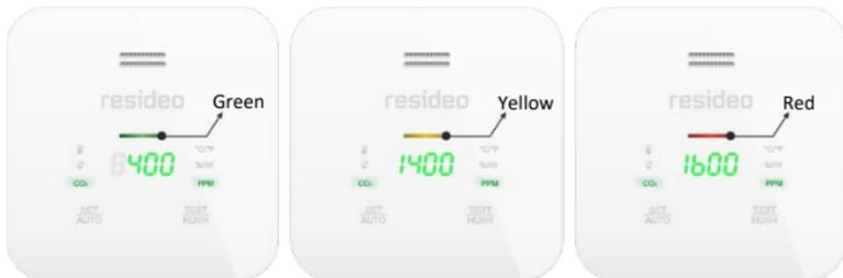
When CO<sub>2</sub> concentration is  $\leq 1000\text{PPM}$ , the status indicator turns green.
