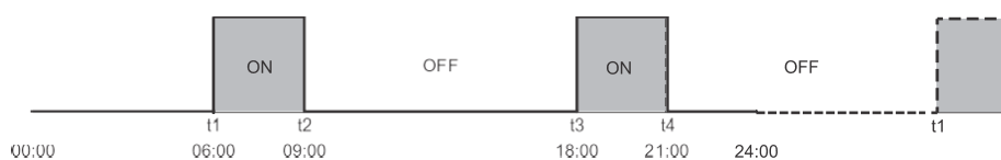
Figure 13: Example of setting the timer – radiator heating
