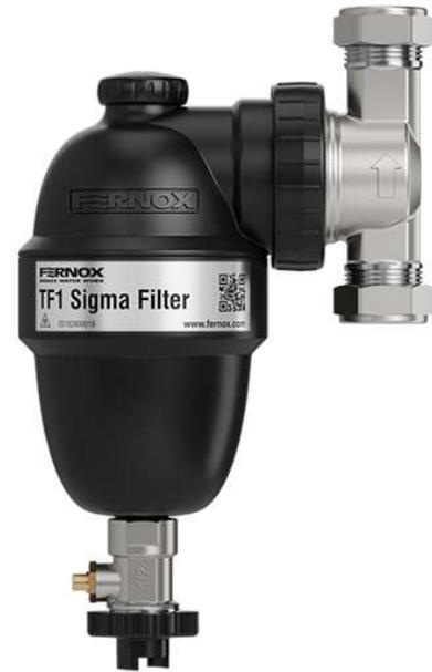
A high-performance, magnetic in-line system filter, the TF1 Sigma Filter is ideal for restricted spaces as it is capable of multiple orientations. This simple to install, composite plastic filter fits onto vertical and horizontal pipework, and works by allowing hydrocyclonic action to deliver contaminants to the unit's powerful magnet assembly for safe removal.
