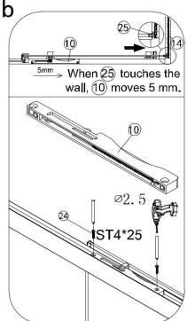
As shown, the second piston is located at the top of the fixed glass profile frame, located at 25 against the glass
