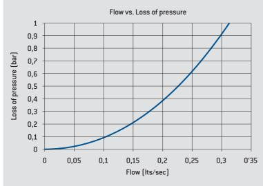
Hydraulic characteristics obtained according to EN 1267.
