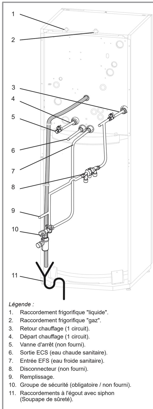
figure 28 - Raccordements
