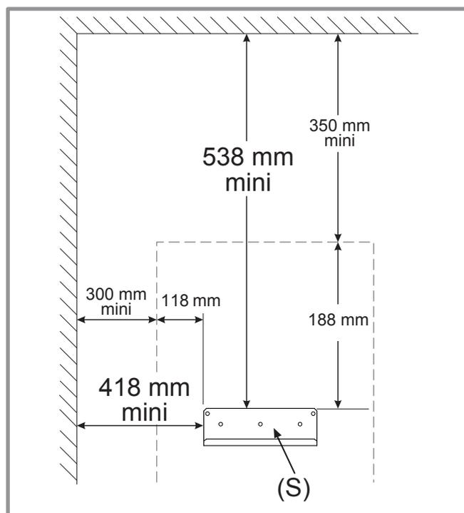
figure 15 - Fixation du support
