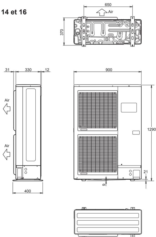
figure 1 - Dimensions en mm
