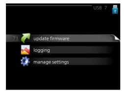
In menu 7.1 on the indoor module/control module, the following software updates can be performed:
