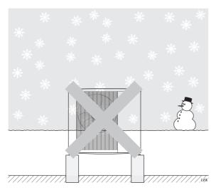
Prevent snow from building up and covering the grilles and drain holes on F2120.
