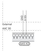
At 0 V the shunt is closed and at 10 V the shunt is open.
