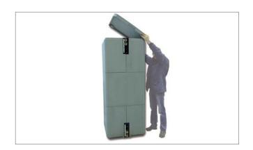
**6)** As a next step, the two upper insulating shells must be removed. Make sure to remove these at an angle (about 45°). This task should be done by two people to ensure that the insulating shells are not damaged.
