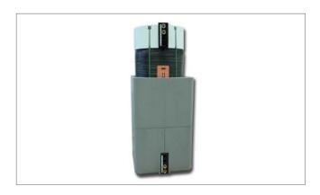
8) Lift the two middle shells slightly to allow the tongues of the lower shells to detach from the grooves in the middle shells. Both of the middle insulating shells can now be pulled away.
