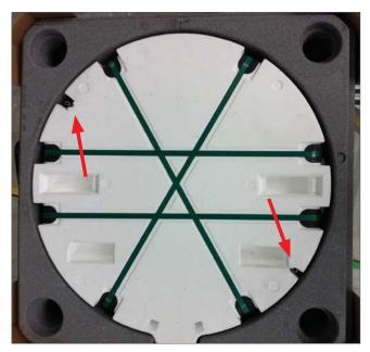
6) The procedure for fitting the sensor from below is exactly the same. The sensor must first be inserted into the rubber feedthrough in the connection panel from the outside. The cable is then fed along the white foot part to the sensor sleeve. The sensor can then be fed into the sleeve at the required height from below.
